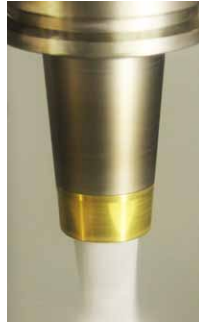
COOLCAP® in action: uniform, ring-shaped cooling jet
